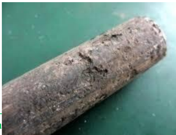
Figure 3. Corrosion damage to downhole components of a sucker rod pump.
