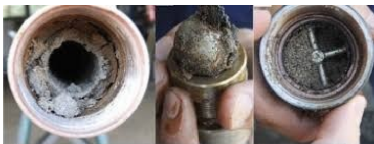
Figure 2. Sand accumulation in the sub-packer plunger.
