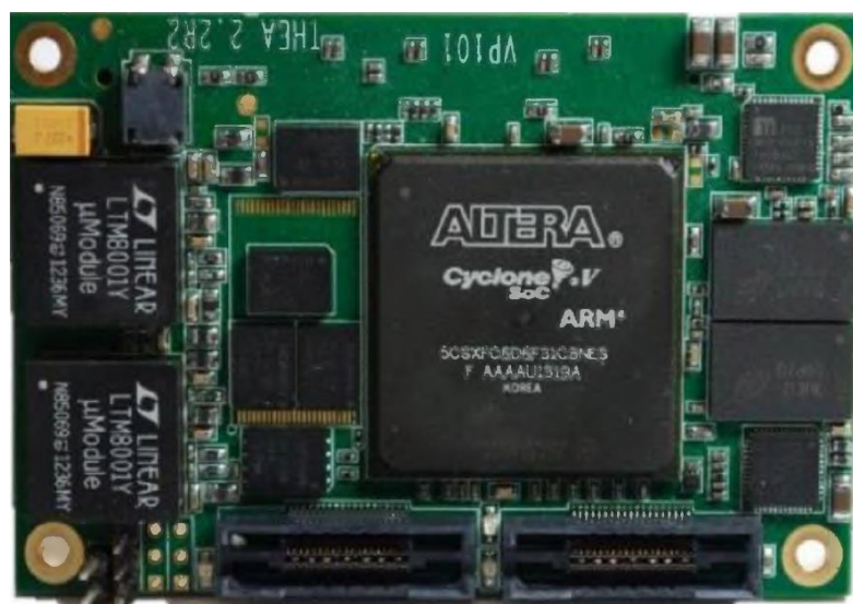
Figure 1 – Receiver Unit of the Automatic Dependent Surveillance (ADS) System
